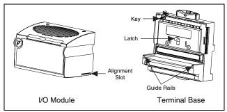
Figure 1. Installing the FP-CTR-502
